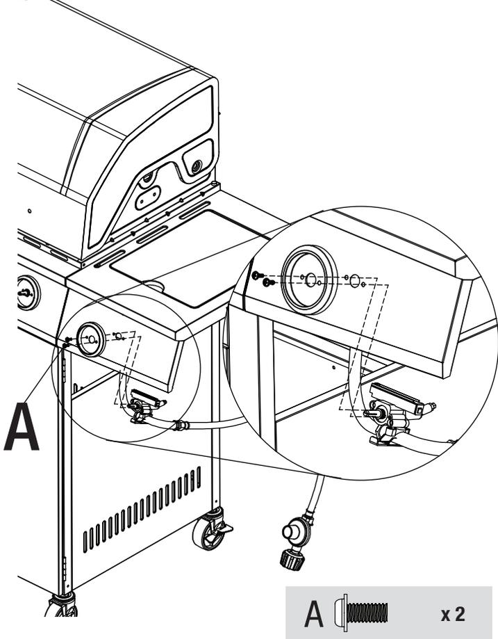
**18** Insert Side Burner, Side Burner Grid and Igniter Wire
